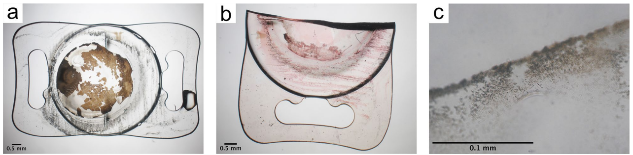
Figure 3. Light microscopy investigation of IOL 3a. Light microscopy (a) shows flat and granular deposits on the IOL's surface. Alizarin Red (b) and Von Kossa (c) staining reveal the deposits had formed on the surface (b) and within the IOL polymer (c) and consist of calcium phosphate.
