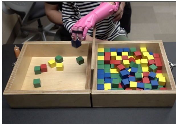
Figure 3. Box and Block test used to test gross manual dexterity being performed by the affected hand. Tasks will involve moving as many blocks as possible from one side of the partition to the other in one minute.
