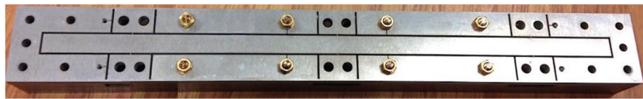
Figure 5. A free-hinged-hinged-hinged-free beam made by precision EDM process. The whole structure is wire cut with about 3–5 microns tolerance from a single piece of flat metal foil. In this case, the hinges represent micro-pivots of an optimum cross section connecting the middle flexible section (ribbon) to the rest of the frame. Material shown is a composite Tungsten/Copper alloy.
