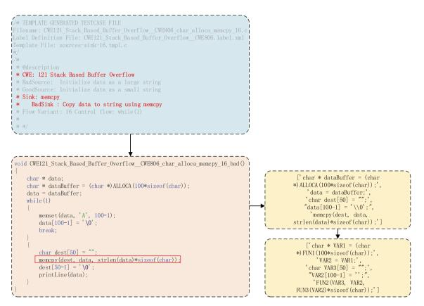
**Figure 2.** The example of extracting code gadgets. To illustrate the extraction of code gadgets, we choose CWE121\_Stack\_Based\_Buffer\_Overflow\_\_CWE806\_char\_alloca\_memcpy\_16.c as an example. In the flowchart, we generate code gadgets by slicing the relevant code according to the API functions and dealing with standardized processes.
