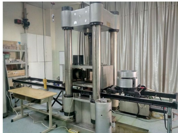
(a) RLJW-2000 rock mechanics test system (b) Sketch of loading device
