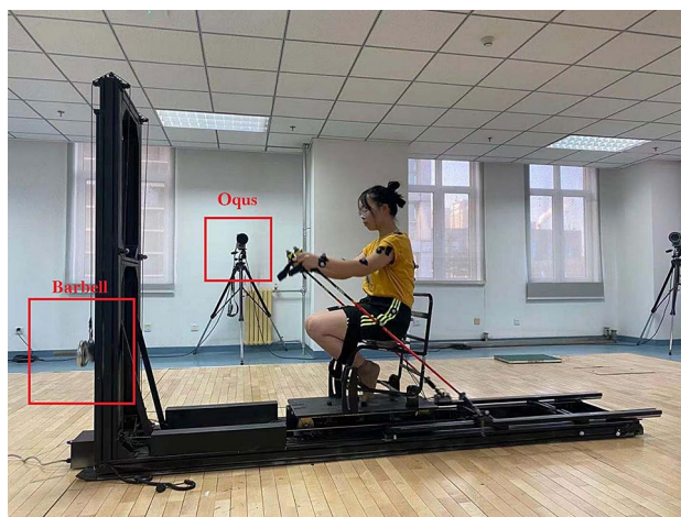
Figure 2. Illustration of the experimental setup during the simulation of cross-country sit-skiing double poling process.
