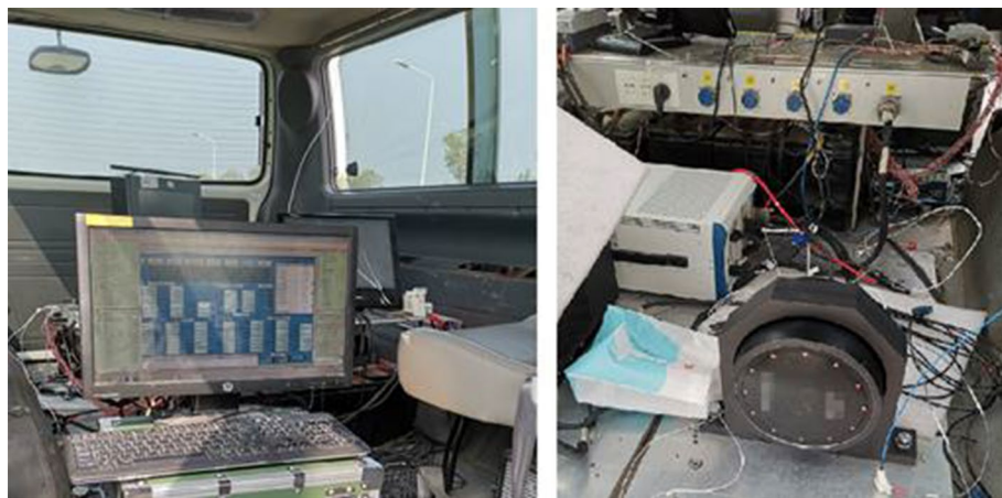
Figure 6. SINS/BDS integrated navigation system and test equipment.
