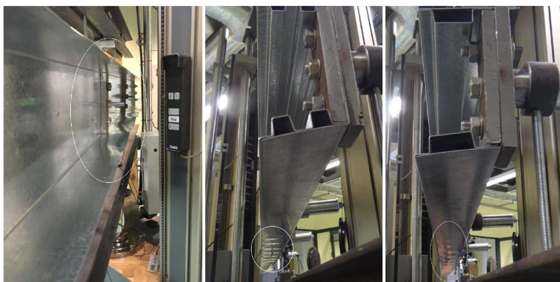
Figure 8. C-Shape no reinforced, double box flange and one box beam after loss of stability.
