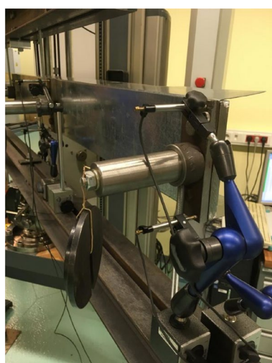
Figure 7. Displacement sensors applied to four points of stiff steel plates.
