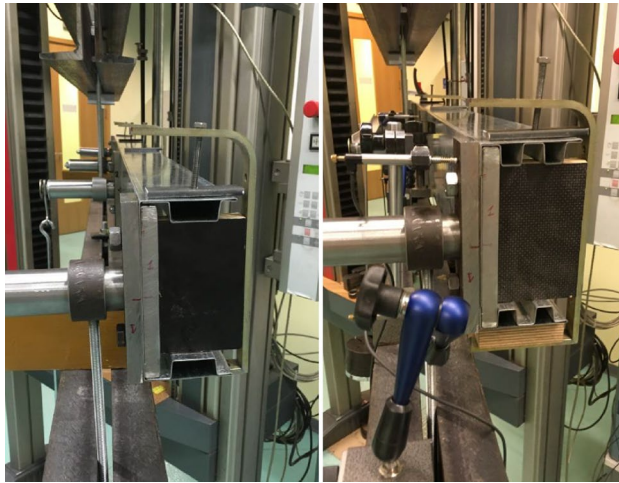
Figure 14. Tested members with plywood diaphragms.
