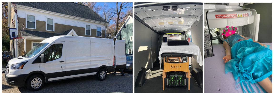
Figure 2. Timeline of scanning from arrival at the participant's home (left), set up of the scanner bed and powering on of the system using the portable battery supply (middle), and finally scanning of the participant (right). Informed consent and assent was obtained to take, use, and publish these photos of their home and participating child in print and online open-access publications.
