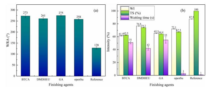
Figure 5. The WRA (a), WI, TS and wetting time (b) of the finished fabrics.
