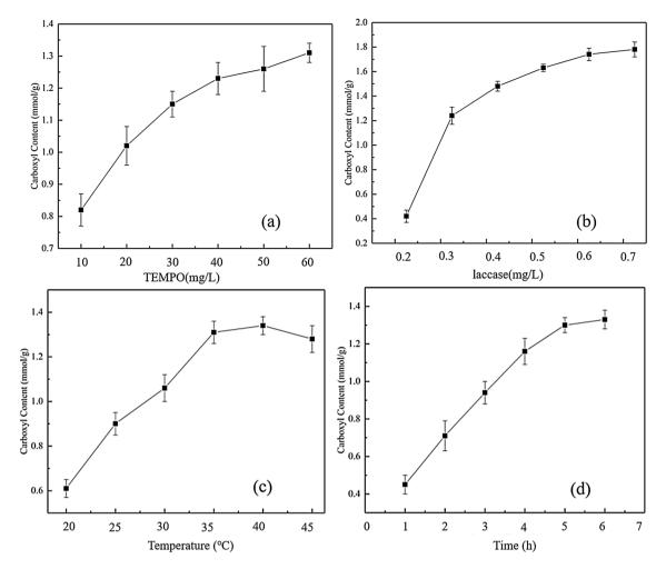
**Figure 1.** Effect of TEMPO factor (**a**), laccase factor (**b**), reaction temperature (**c**) and reaction time (**d**) on the carboxyl content of openSu.
