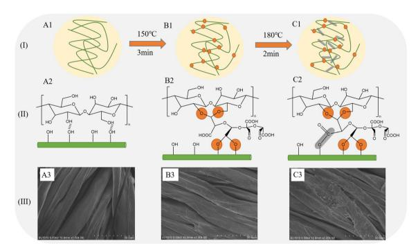
**Figure 7.** Possible reaction mechanism (I, II), SEM images (III) of reference (A1, A2, A3), openSu (150 °C) (B1, B2, B3) and openSu (150 °C and 180 °C) (C1, C2, C3).
