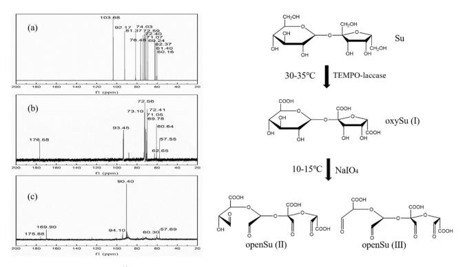
**Figure 3.** <sup>13</sup>C NMR spectra of sucrose (**a**), oxySu (**b**) and openSu (**c**) and the oxidation process of sucrose.
