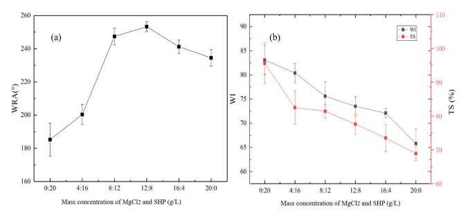
**Figure 4.** The effects of different mass concentration ratios for  $MgCl_2$  and SHP, on the WRA (**a**), WI and TS (**b**) of the finished fabrics.
