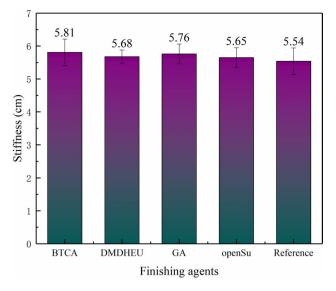
Figure 6. The stiffness of the finished fabrics with different finishing agents.
