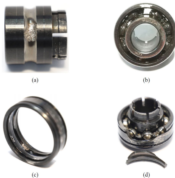
Figure 13. Failure bearings: (a) inner race wear; (b) cage fracture; (c) outer race wear; (d) outer race fracture.
