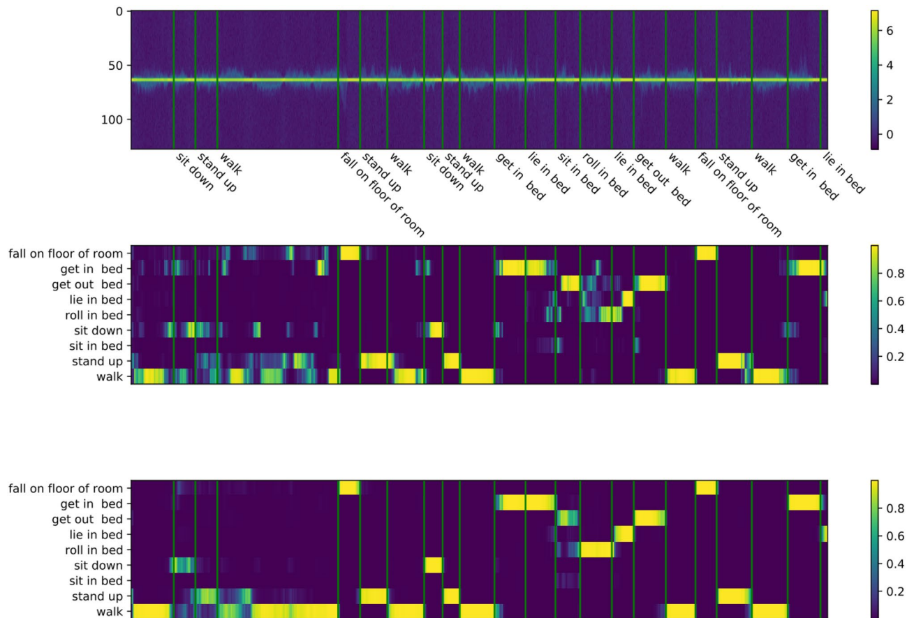
Figure 1. (Top) MD signatures over time in dB (middle) unidirectional RNN over time with classes on the y axis with activities annotated with vertical green lines. The color scale visualizes the confidence \in [0, 1] of the model in a class. (Bottom) Bidirectional RNN over time with classes on the y axis. The color scale visualizes the confidence \in [0, 1] of the model in a class.
