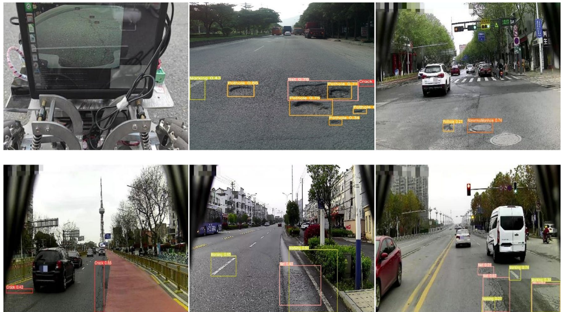
Figure 15. The deployment of the improved YOLOv5s in a self-built mobile platform and its object recognition results.
