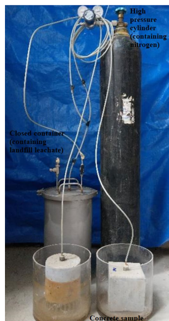
Figure 1. Osmotic pressure device.
