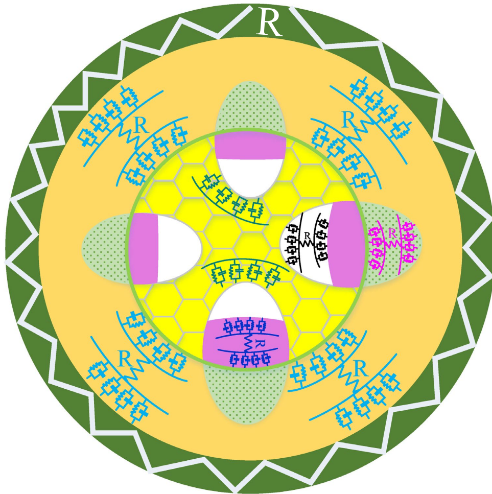
Figure 3. Plant stem electrical equivalent circuit. The epidermis is a single protective hard layer represented with a resistor. While, the cortex and vascular bundle elements consist of a membrane and inner fluid responsible for storing carbohydrates and the flow of water, nutrients, food, and organic materials represented by a resistor and a fractional-order capacitor. The pith is a spongy structured tissue described by a fractional-order capacitor.
