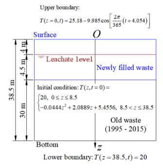
Figure 1. Physical model for heat transfer in the Wuxi landfill.
