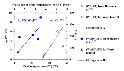
**Figure 3.** Method of empirical fitting for  $A_T$  and  $B_T$ .
