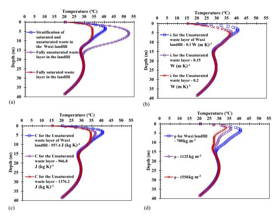
**Figure 5.** Comparison of the temperature distribution on Day 365 under the conditions of the different sensitive parameters: (**a**) stratification of the saturated–unsaturated waste; (**b**) heat conductivity of the waste ( $\lambda$ ); (**c**) specific heat capacity of the waste (*C*); (**d**) density of the waste ( $\rho$ ).
