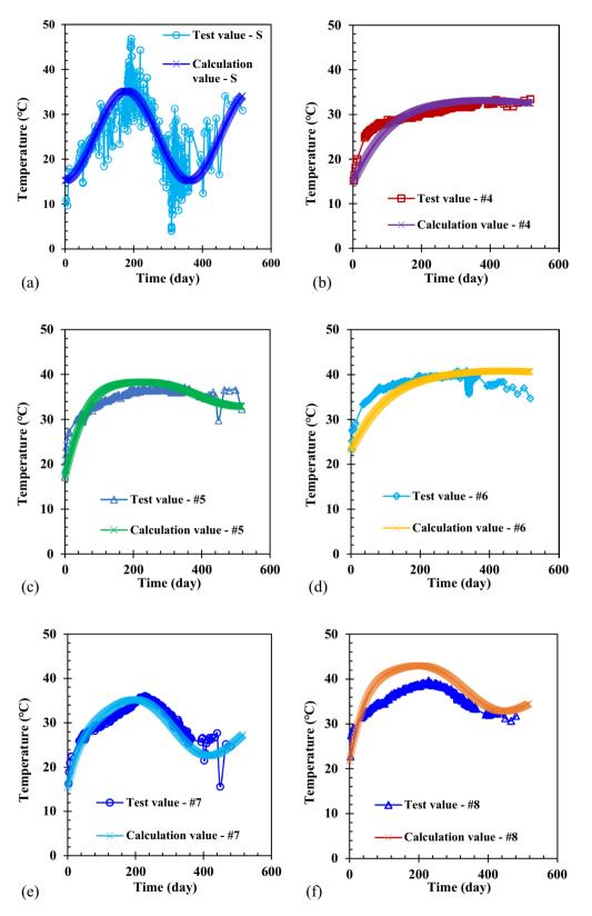
**Figure 2.** Comparison of the calculation and test values of temperature with time at the bottom of the different wells: (**a**) Surface (Depth: 0 m); (**b**) #4 well (Depth: 5.88 m); (**c**) #5 well (Depth: 3.58 m); (**d**) #6 well (Depth: 6.56 m); (**e**) #7 well (Depth: 1.34 m); (f) #8 well (Depth: 2.05 m).
