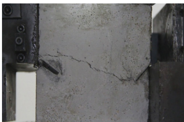
Figure 24. Photograph of a specimen showing fractures propagation.
