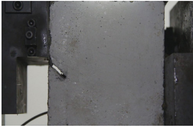
Figure 16. Photograph of a specimen showing fractures appearing from the left boundary of the rock mass.
