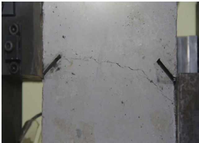
Figure 28. Photograph of a specimen showing fractures propagate in the middle of the rock mass.
