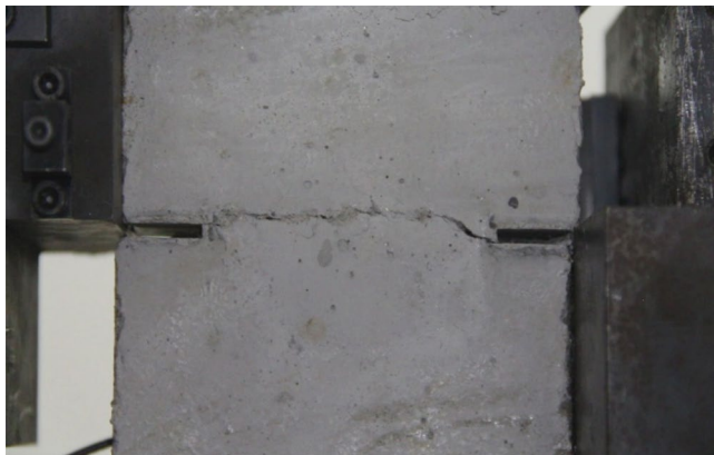
Figure 60. Photograph showing penetration patterns of the tip of the left crack and the tip of the right crack are directly connected.
