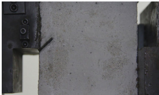
Figure 43. Photograph of a specimen showing fractures appearing in the middle of the specimen.
