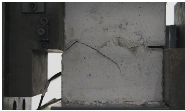
Figure 64. Photograph showing penetration patterns of the tip of the left crack and the tip of the right crack indirectly expand and connected.
