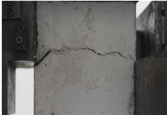
Figure 42. Photograph of a specimen showing fractures penetration.
