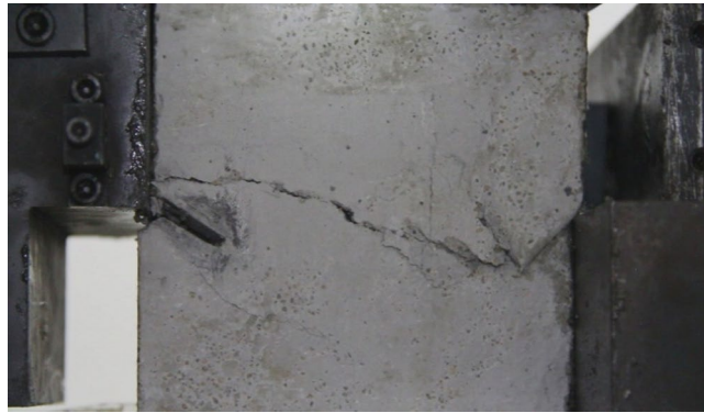
Figure 63. Photograph showing penetration patterns of the left boundary and the tip of the right crack are connected.
