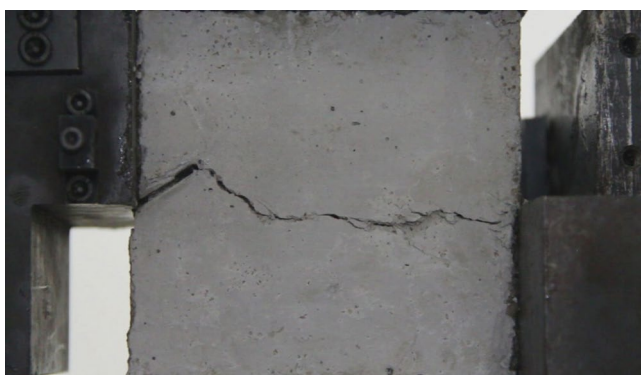
Figure 61. Photograph showing penetration patterns of the tip of the left crack and the right boundary are connected.
