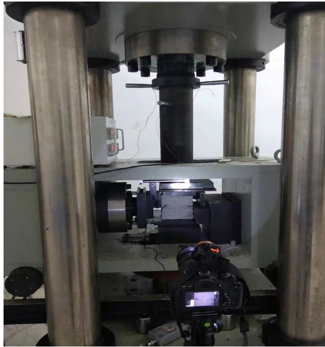
Figure 3. Photograph of the compression shear test showing a specimen ready to be tested.
