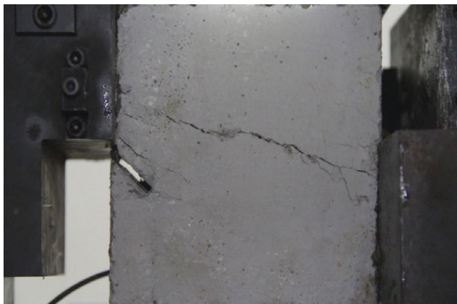
Figure 17. Photograph of a specimen showing fractures penetration.
