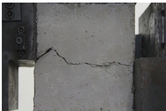
Figure 40. Photograph of a specimen showing fractures penetration.
