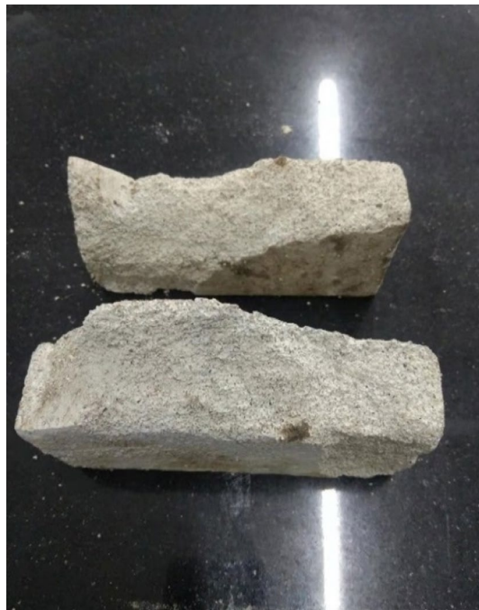
Figure 15. The shear fracture surface of the specimen.
