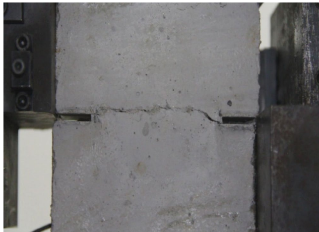
Figure 12. Photograph of a specimen showing fractures penetration.
