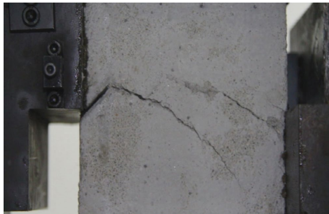
Figure 44. Photograph of a specimen showing fractures propagating and penetration.
