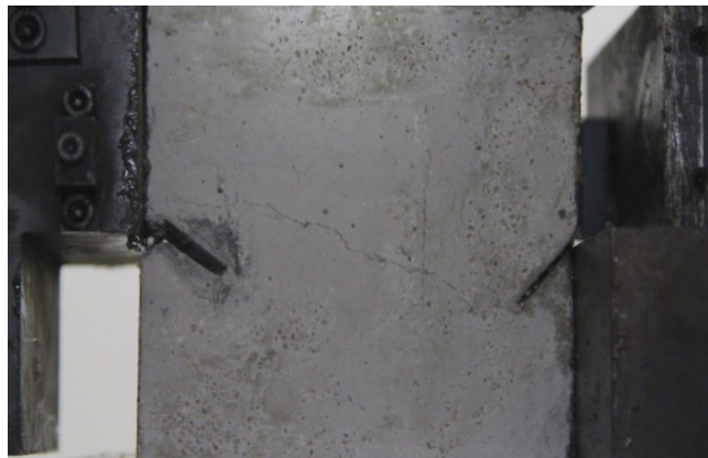
Figure 23. Photograph of a specimen showing fractures appearing in the middle of the rock mass.
