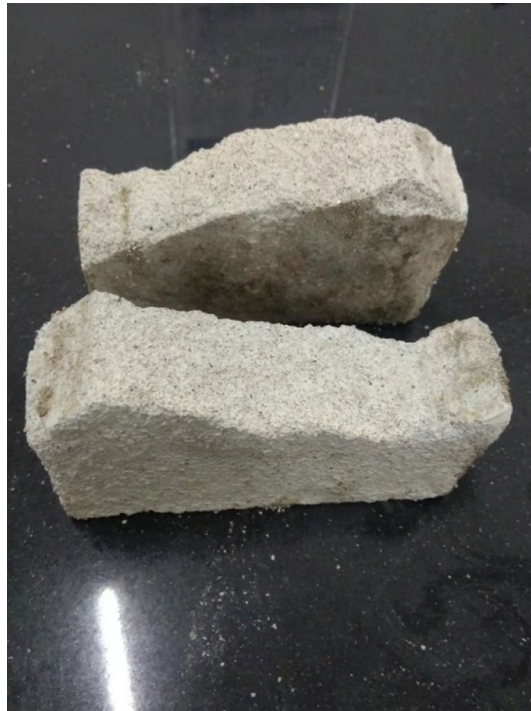
Figure 22. The shear fracture surface of the specimen.
