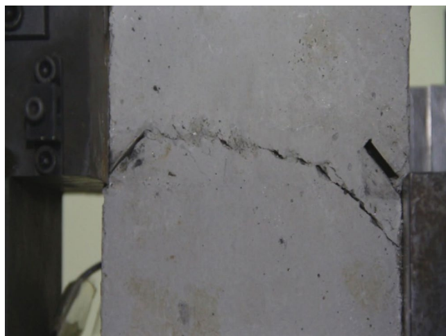
Figure 30. Photograph of a specimen showing fractures penetration.
