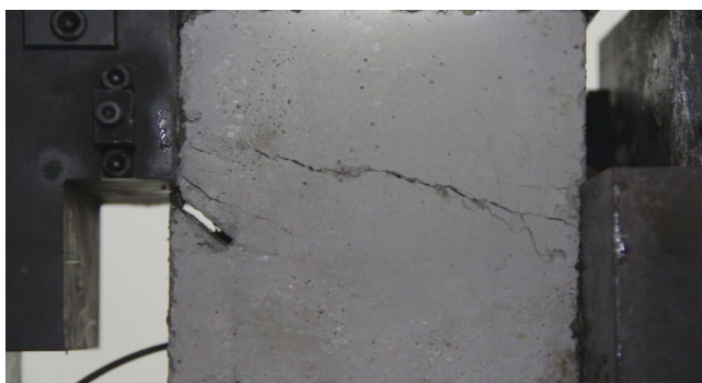
Figure 62. Photograph showing penetration patterns of the left boundary and the right boundary are connected.
