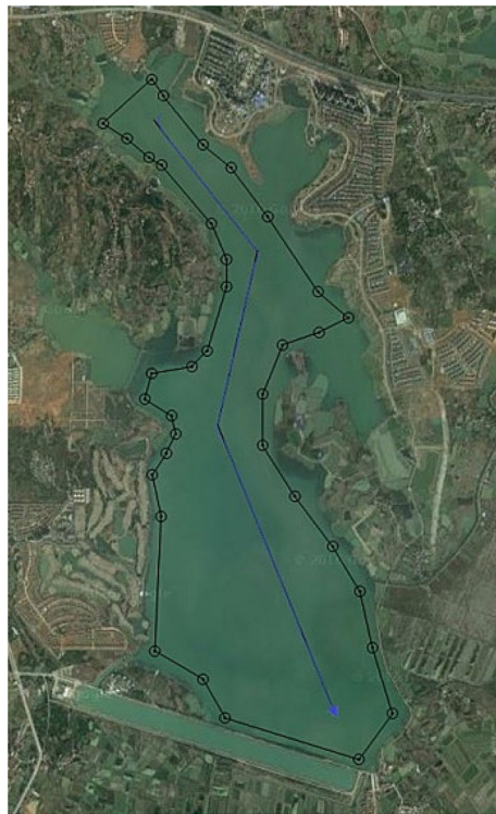
Figure 12. Sturgeon' USV path following test result.
