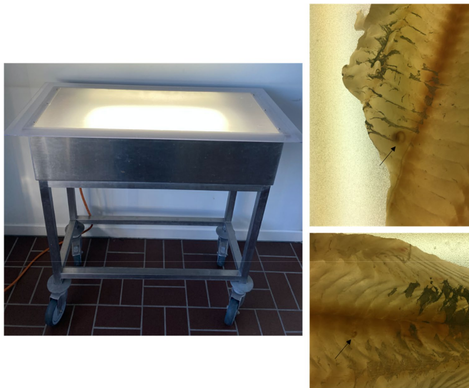
Figure 2. The candling table (left) and examples (right) of visualised embedded ascaridoid larvae in fish muscles (arrow) placed on the candling table.
