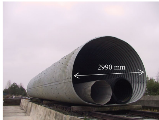
Figure 11. General view of the tested steel Multi Plate structure including the two pipes from the chapter 2.1.
