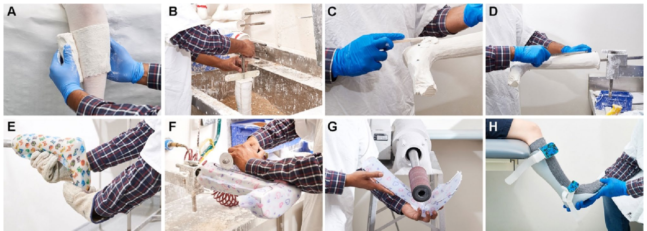
Figure 1. Traditional AFO fabrication involving plaster moulding. (A) Creating the negative cast of a person, (B) filling the negative cast with liquid plaster to produce the positive cast, (C) applying additional plaster modifications, (D) refining plaster modifications, (E) vacuum forming polypropylene over modified cast, (F) cutting the polypropylene AFO from the cast, (G) finishing the AFO and (H) fitting the AFO to a person.
