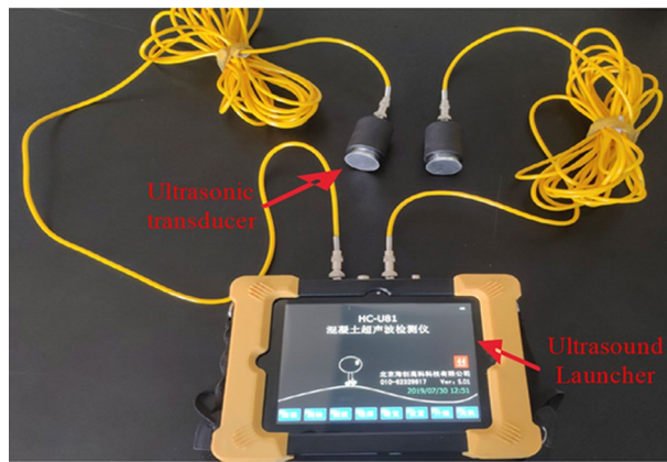
Figure 6. Ultrasonic wave velocity testing system used in this study.
