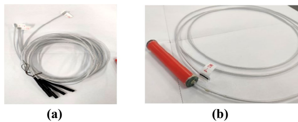
Figure 7. Experimental cartridge production system with (a) detonator, and (b) blasting cartridge.
