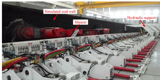
Figure 9. The mechanical testing and analysis experimental platform for fully mechanized working face.
