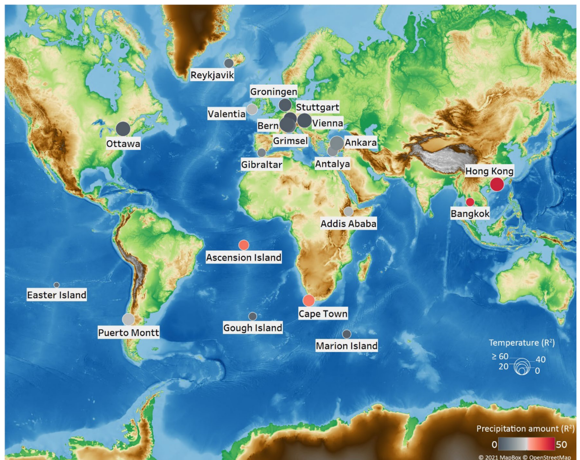
Figure 1. The location of long-term GNIP stations and the coefficient of determination ( R^2 ) of \delta^{18}\text{O} – T and \delta^{18}\text{O} – P nonparametric relationships. Base map is from OpenStreetMap and OpenStreetMap Foundation under the Open Database License ( https://www.openstreetmap.org/copyright ).
