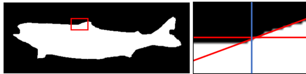
Figure 5. Localization of the upper fin beginning. Left—Segmented fish with selected region of upper fin beginning. Right—Magnification of selected region; blue line—horizontal center of the image, red lines—lines fitted to the left and right halves of the border pixels. Produced by Matlab R2020b.
