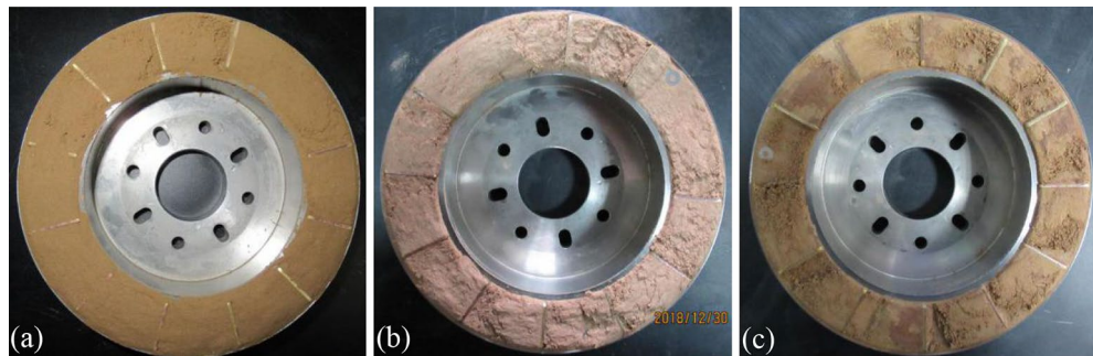
Figure 4. Shear planes of specimen after ring shear tests. (a) Loess; (b) red clay; (c) LRCI.
