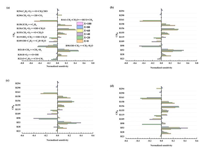
**Figure 8.** Normalized methane sensitivity coefficients for four equivalent ratios [(a)  $\Phi = 0.8$ , (b)  $\Phi = 1.0$ , (c)  $\Phi = 1.2$ , (d)  $\Phi = 1.4$ ] during explosion.
