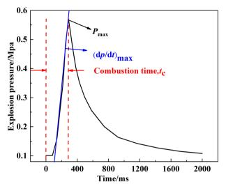
Figure 2. Typical pressure trajectory during an explosion.
