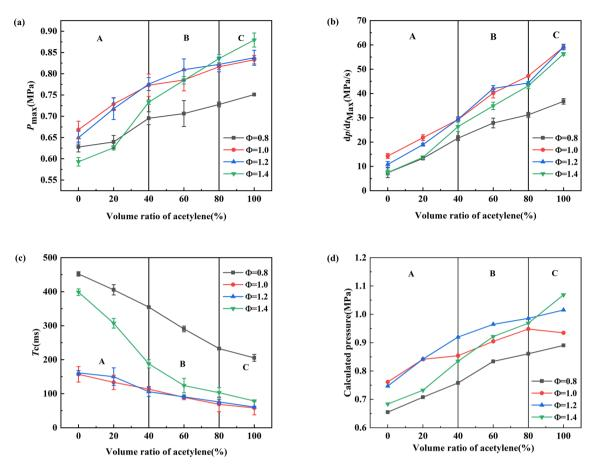
**Figure 6.** Explosion parameters for a methane–acetylene–air mixture [(a)  $P_{\text{max}}$ , (b)  $(dP/dt)_{\text{max}}$ , (c)  $T_c$ , and (d) calculated pressure].
