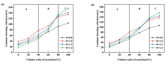
**Figure 7.**  $S_L$  value of mixed gas [(a)  $S_L$  from spherical flame method, (b)  $S_L$  from GRI Mech 3.0].
