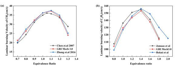
Figure 3. Laminar burning velocity verification [(a) methane, (b) acetylene].
