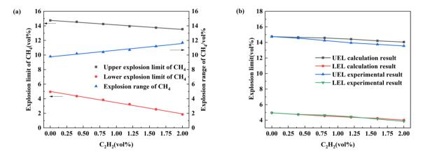
**Figure 4.** Explosion limit for methane in air [(**a**) Methane explosion limit change, (**b**) comparison of calculated and experimental values].
