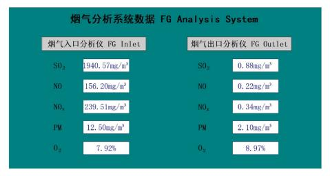
Figure 15. Inlet and outlet flue gas composition monitored by online CEMS system.
