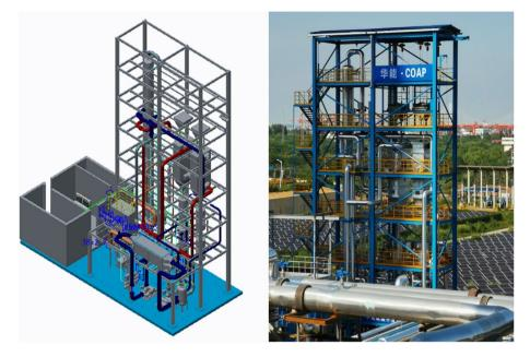
Figure 13. 3D model (left) and a photo (right) of the pilot test platform.
