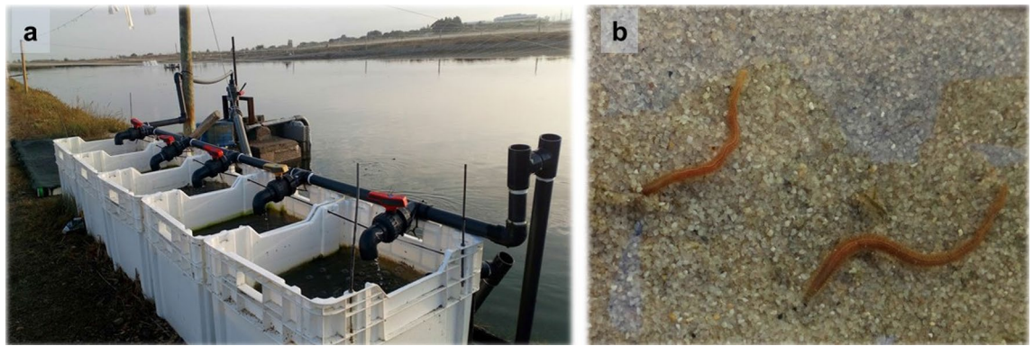
Figure 5. (a) Polychaete assisted sand filters (PASF) used in the present study; (b) Hediste diversicolor in sand bed.
