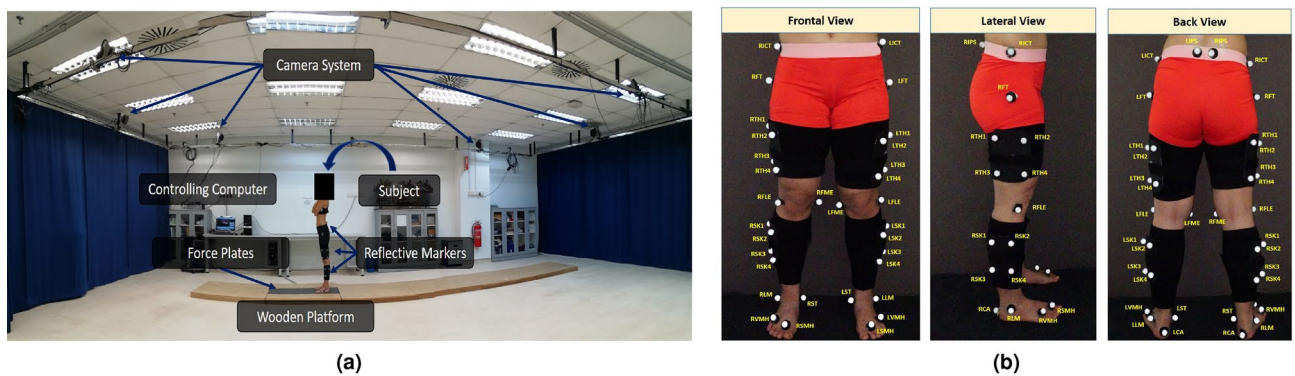
Figure 4. Data Collection Process (a) Laboratory setup with six motion cameras (ProReflex MCU, Qualisys, Gothenburg, Sweden) for joint motion measurements, two force plates (Bertec, type FP 4060-07, Bertec Corporation, OH, USA) embedded on to a 10m long wooden platform for vGRF measurements. (b) Marker placement with 36 markers recommended by Visual3D (C-motion Inc., Kingston, Canada). Double-sided adhesive stickers were used to stick markers on the segments and joints. Cluster markers with four individual markers were attached to each shank and thigh segments. Cluster markers were tighten using a stretchable band, to ensure no errors due to loosening attachments. All markers are labelled with a unique marker name.
