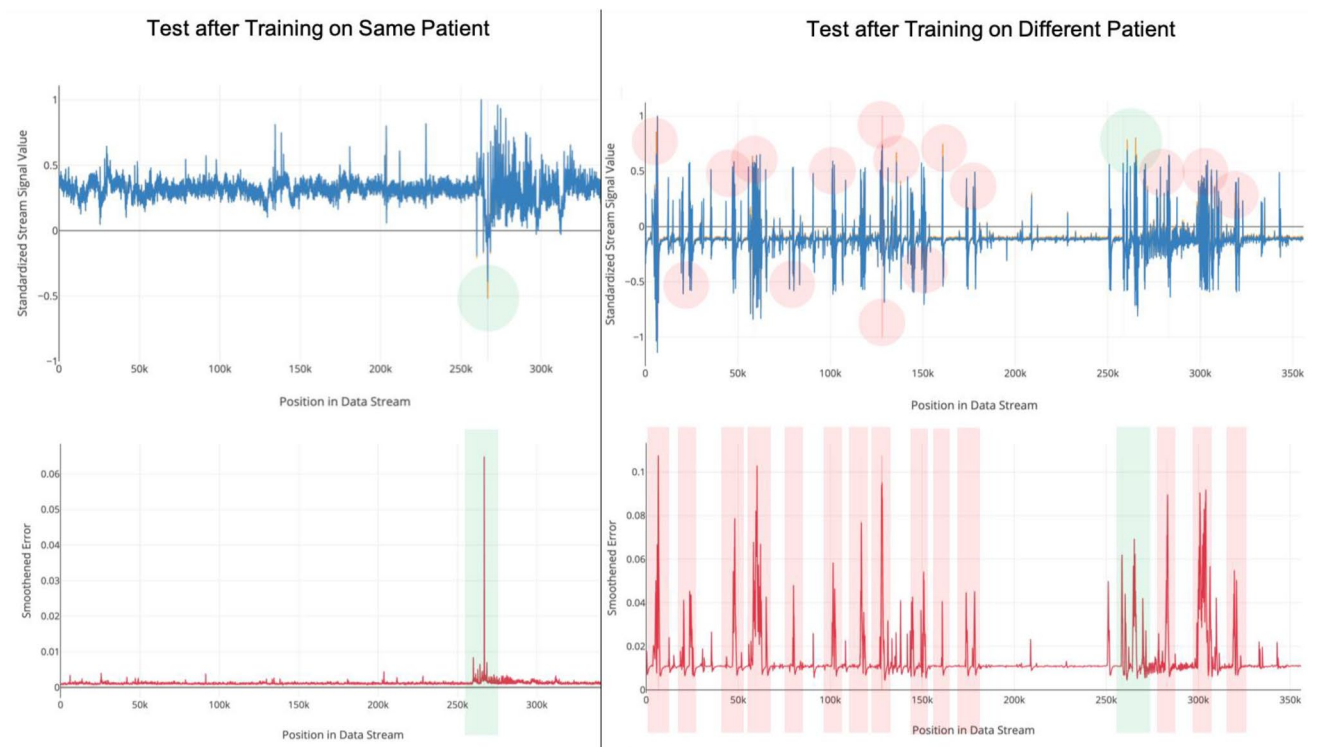
Figure 3. Crossover testing produces a large increase in the number of false positive results. This indicates that trained models are attuned to the unique electrical signal of a given patient. Green shading refers to prediction mismatches that correspond to correctly identified anomalies whereas red shading refers to prediction mismatches that correspond to false positives.
