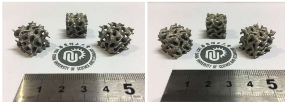
Figure 18. Formed samples of Gyroid complex surface.
