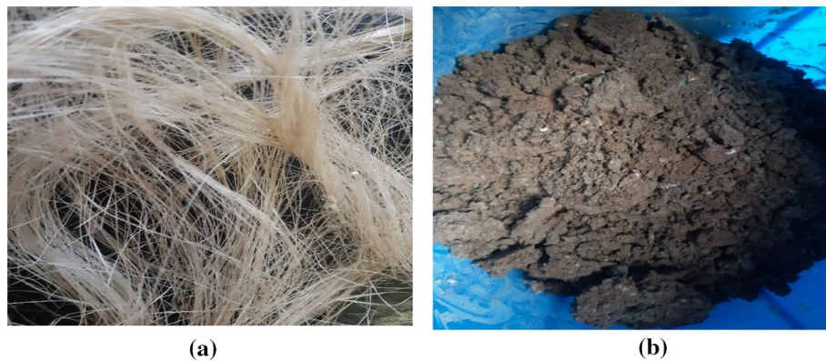
Figure 1. Image of materials used in the study (a) banana stem fiber (b) cement–sand–paper slurry.
