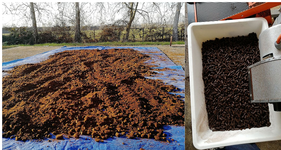
Figure 1. Spent coffee ground (SCG) before (left) and after (right) the pelletizing process.
