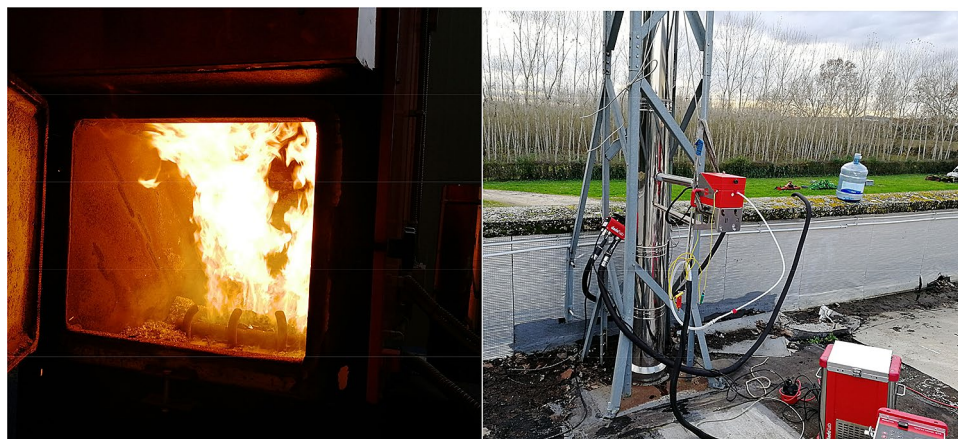
Figure 2. Combustion chamber (left) and probe system for sampling on the stack (right).
