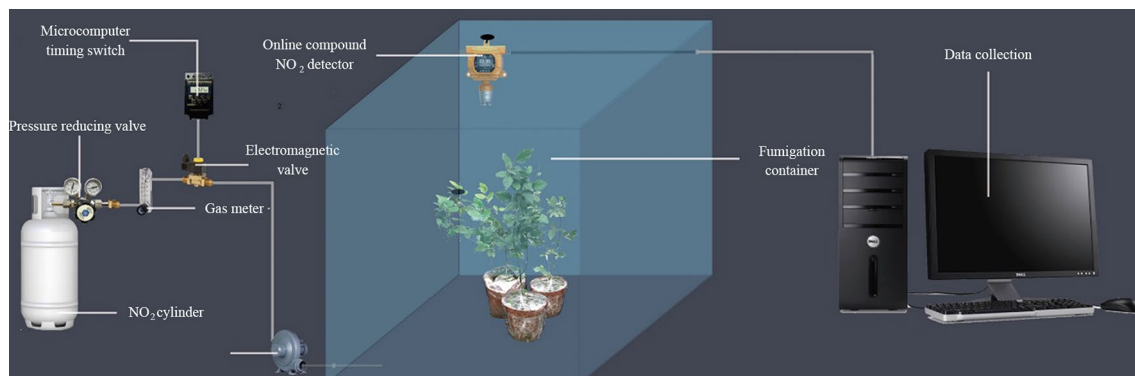
Figure 7. The fumigation test device for timing regulation and recording of the \text{NO}_2 concentration (drawn with Adobe Photoshop CC2019; https://download.zol.com.cn/tuiguang/detail/46/456409.shtml?qw= ).
