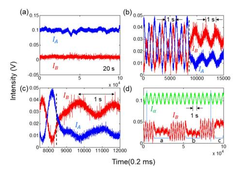
**Figure 3.** Experimental results for USCKD in Fig. 1. (a)  $\psi_{12} = \varphi_{12}$ . (b) Switching between CBW and USCKD. (c) expansion of (b). (d) Conventional MZI output (green) vs. CBW [USCKD(a/b/c)] (red). In (b) and (c),  $\varphi_{12} = -\psi_{12} = 1Hz$  before the dashed line;  $\varphi_{12} = \psi_{12} = 1Hz$  after the dashed line. The value of vertical axis is arbitrary.
