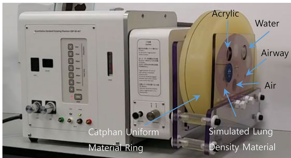
Figure 1. Experimental set-up of the COPD gene phantom. It was attached to the QSP actuator.
