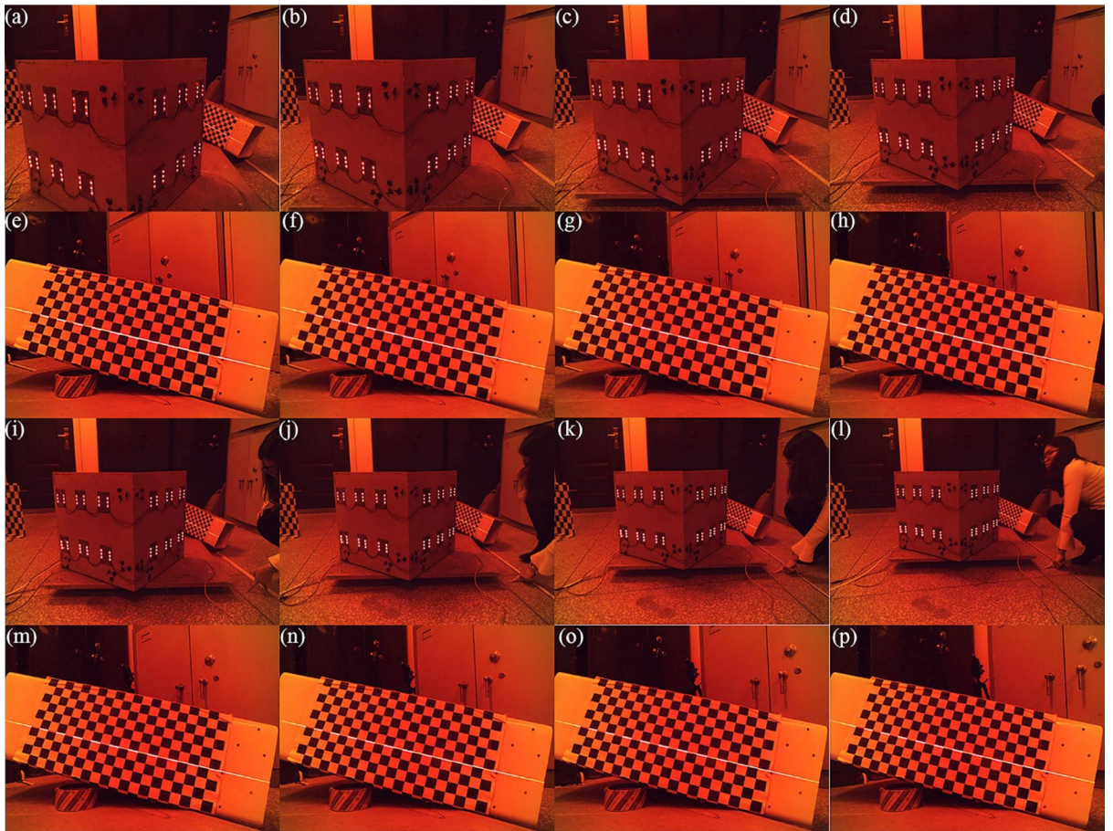
Figure 3. Experimental images of the internal and the external cameras. (a–d) the experimental images of the external camera. The camera-board distances are 600, 700, 800, 900 mm. (i–l) the experimental images of the external camera. The camera-board distances are 1000, 1100, 1200, 1300 mm. (e–h) and (m–p) the experimental images of the internal camera related to (a–d) and (i–l).
