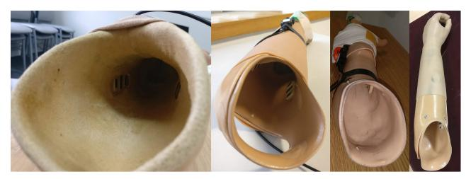
**Figure 2.** Socket mounted electrodes. Images from participants' own clinically prescribed prostheses. Note that in the far-left image, the quality of the skin–electrode interface is disrupted by a leather shim on the interior of the socket.
