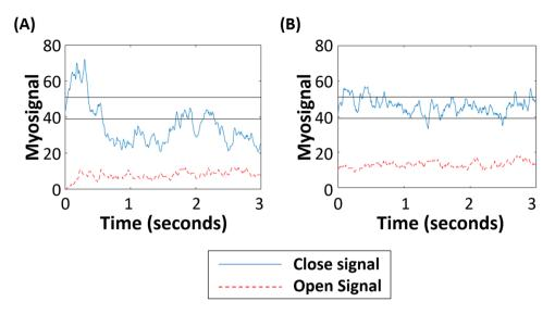
**Figure 8.** Static Tracking Task closing trial example for the (**A**) worst (22%) and (**B**) best (85%) performers. Participants were instructed to keep the blue signal (controlled using the muscle for hand closing) inside the boundary lines, whilst keeping the other muscle (red dotted) relaxed. The trial lasted 3 s.
