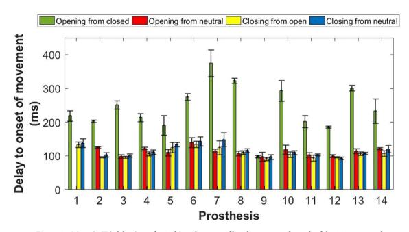
Figure 9. Mean ( $\pm$  SD) delay (out of 5 trials) to the onset of hand movement for each of the 14 user owned prostheses. For all hands except hand 9, the delay to the onset of hand opening from a fully closed position was significantly longer (t-test:  $p \le 0.01$ ) than all other measures of delay. For hand 1, it was not possible to record the delay to the onset of hand opening from a neutral aperture.
