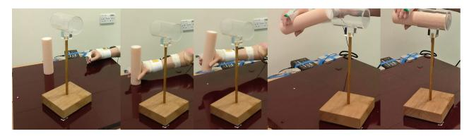
**Figure 5.** Cylinder task, participants were asked to reach to grasp a nylon cylinder with a foam outer surface (diameter 52 mm, length 200 mm, weight 350 g). Lift it and rotate it to the horizontal before placing it into a transparent tube (inner diameter 64 mm, length 100 mm).
