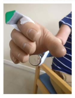
**Figure 3.** 500 g Load added to prosthetic hand. The load was bandaged to the hand at the proximal palm/distal wrist level so as not to disrupt the opening/closing of the hand.
