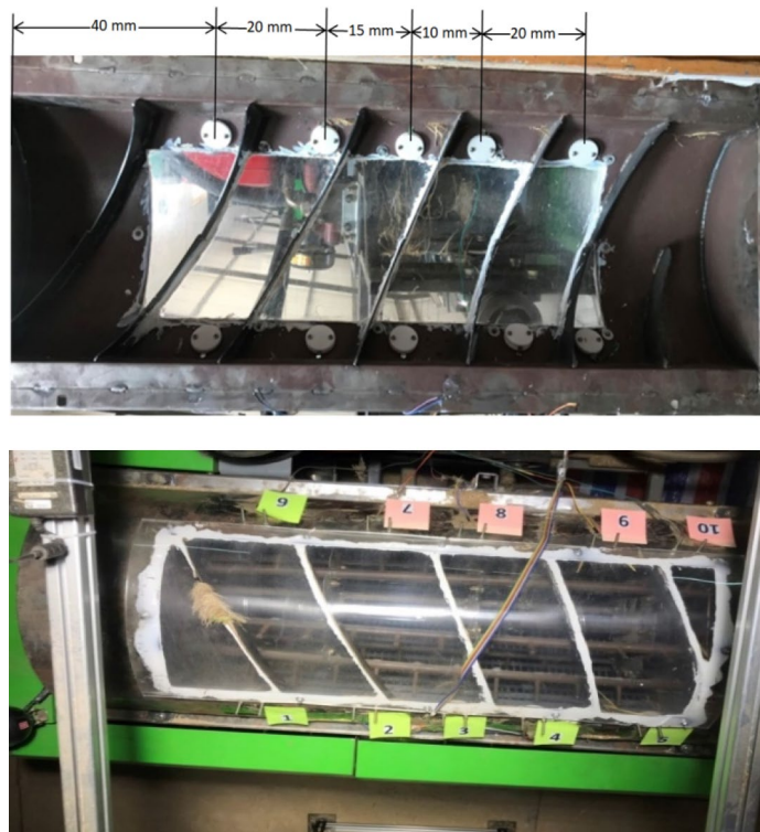
Figure 7. Sensors installation in thresher cover.
