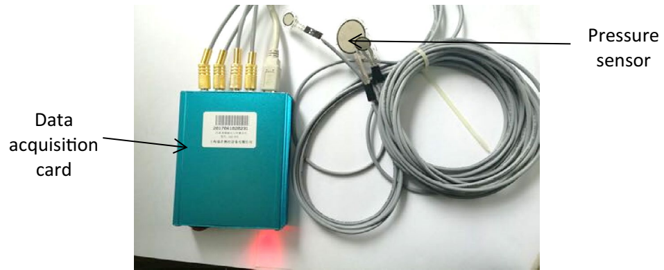
Figure 5. Pressure sensing system.
