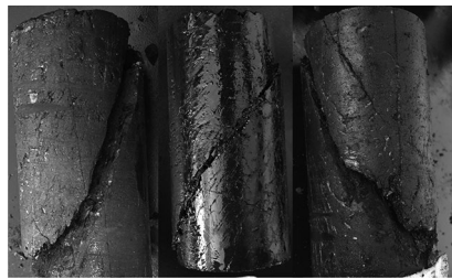
Figure 1. Failure characteristics of coal samples.
