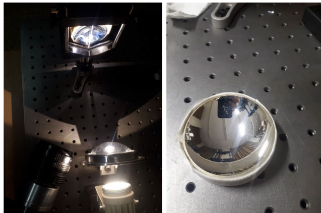
Figure 11. Left: The measurement optical setup. A ribbon of white paper with the size 1.2 \times 70 \text{ mm}^2 is placed close to focal point. The mirror is translated by the micro positioner along the spherical mirror optical axis. Right: silver coated lens spherical mirror.
