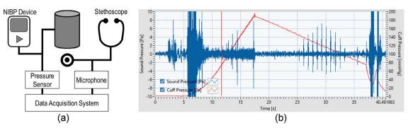
**Figure 1.** Blood pressure data collection system using a stethoscope and data acquisition board: (**a**) data acquisition system and stethoscope connected to a microphone, and (**b**) LabVIEW-based data acquisition software.
