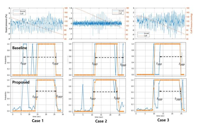
**Figure 10.** Sound signal (top) and predicted probability with the baseline (middle) and the proposed model (bottom) in three noisy cases.
