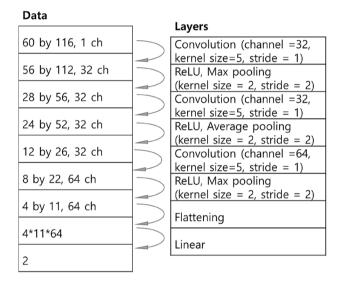
Figure 8. Structure of the CNN model of the baseline method.
