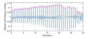
Figure 2. Cuff pressure oscillation for peak extraction.
