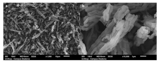
**Figure 6.** Scanning electron microscopy images of SBA-15 (Santa Barbara Amorphous silica) before antigen adsorption in macro pores. (**a**) 1000x magnification; (**b**) 10,000x magnification.
