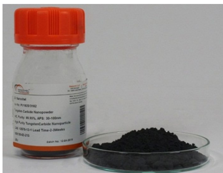
Figure 1. Nanoparticles of tungsten carbide (WC) 13 .
