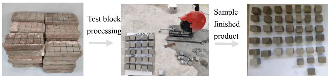
Figures 4–6. Figure 4 Brick samples. Figure 5 Specimen cutting and grinding. Figure 6 Sample finished product.
