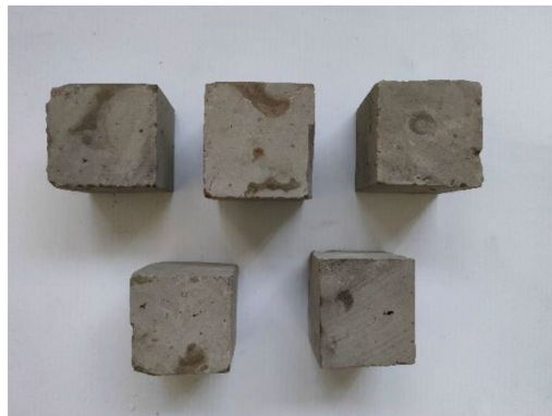
Figure 18. Evidence of sample frosting.
