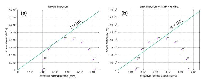
**Figure 7.** Mohr circle graphical representation of the state of stress on individual planes with  $\beta$  angle step size of 10° (violet dots) and its comparison with Mohr–Coulomb shear failure envelope  $\tau = \mu \sigma_n$  (solid green line) for (**a**) the stress state before fluid injection and (**b**) the stress state after fluid injection with a pore pressure increase at the bottom-hole of  $\Delta P_p = 6$  MPa.
