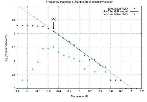
**Figure 3.** The frequency–magnitude distribution (FMD) of the analyzed induced seismicity cluster. The green line indicates the fit of the Gutenberg-Richter model over the local magnitude range  $Mc \le Ml \le 0.5$ , where Mc = -0.5 is the completeness magnitude. The dashed green line is the extrapolation of the Gutenberg-Richter model for the higher and the lower local magnitude values. Circles and diamonds represent the cumulative and the noncumulative FMD, respectively.
