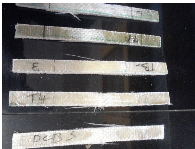
Figure 4. Tearing behaviour of the composite specimen under tension.
