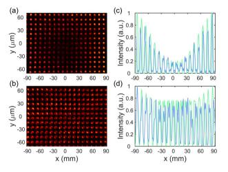
**Figure 7.** Illustration of the self-healing effect. Experimental intensity profiles for the optical vortex (l = +1) at (**a**)  $1Z_T$  and (**b**)  $4Z_T$  and corresponding calculated (green) and measured (blue) intensity distributions in the transverse direction. The plots in (**c**, **d**) corresponds to the plots in (**a**, **b**), respectively.
