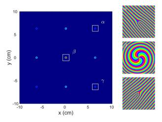
**Figure 4.** Calculated far-field diffraction pattern (left plot) at the distance 1 m and phase profiles for specific diffraction orders (right column) shown by squares in the left plot (l = +3).
