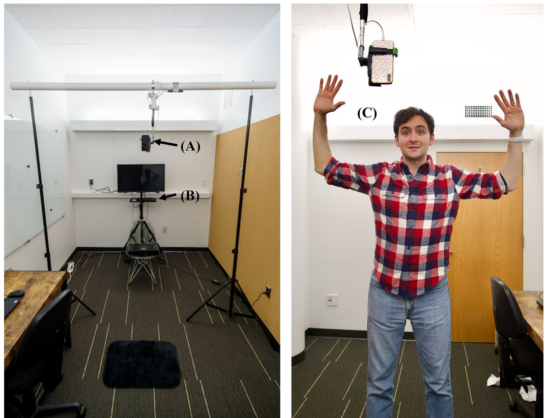
Figure 3. Configuration of study room (left): (A) iPhone XS for facial tracking, (B) Kinect for Xbox One for body tracking, (C) person being tracked during visual referential task.
